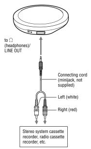
You need to change the setting for "AUDIO OUT" in the OPTION menu so that sound is output to the connected device. The settings of "AUDIO OUT" are shown below. To make those settings, see \* page 26, 28.
